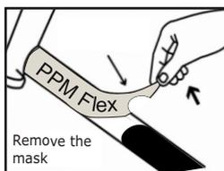
After curing peel of the mask. In some cases it's more suitable to do this when both, surface and mask are still warm.
