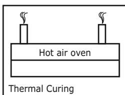
Cure the surface with the mask on it, at the temperature which is needed to cure the paint correctly.
