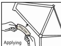
Peel the mask from the paper liner and apply it on the surface which must be covered. Be sure that especially the edges are applied without any air bubbles or tearings.
