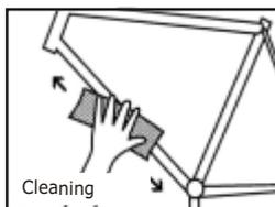
Be sure that the object has a minimal temperature of 16 degrees and the surface is clean, free from dust, grease and oxidations. To avoid problems you may use a degreaser like IPA or an other degreaser who's friendly for the used powdercoat finish.
