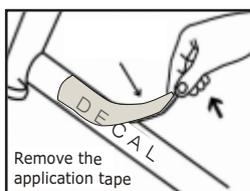
Remove the application tape under a sharp angle. Inspect the decal if it is placed correctly and without airbubbles. In case of bubbling you may use a needle to prick them away. If this brings no solution then check if there is no dust or whatever between the surface and the decal. To improve the adhesion you may heat the decorated surface for at least 30 seconds on an object temperature of 60 degrees.
